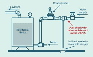
Boilers with chemical additives require an ASSE #1013 – Reduced Pressure Principle Backflow Prevention Assembly.
