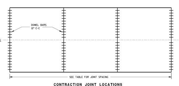
JOINT DETAIL STANDARD DETAIL MODIFIED **URBAN DOWELED**
