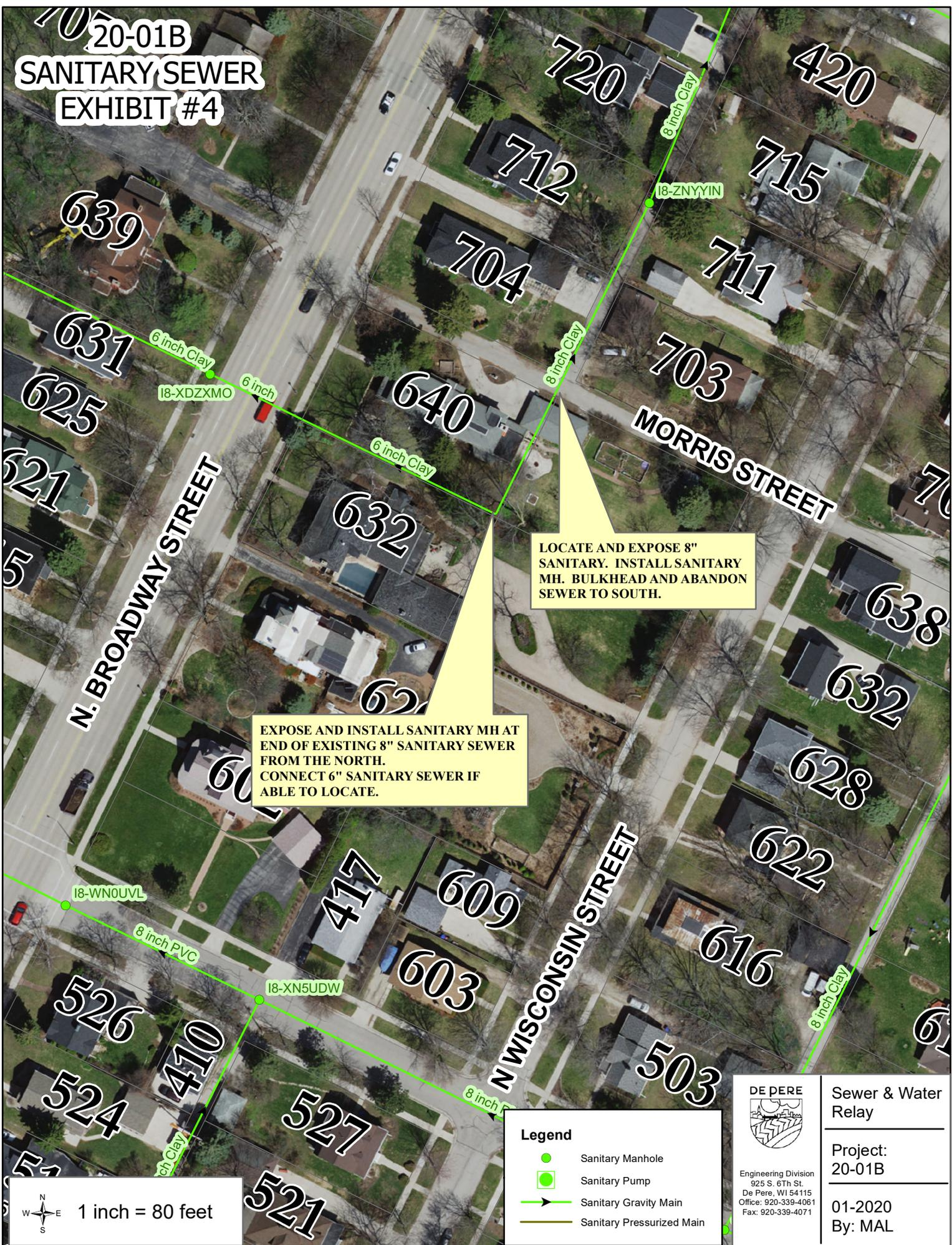
LOCATE AND EXPOSE 8" SANITARY. INSTALL SANITARY MH. BULKHEAD AND ABANDON SEWER TO SOUTH.
