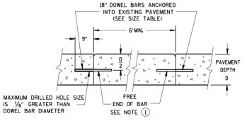
SECTION D-D (FOR 11' LANE WIDTH REDUCE CENTER SPACE TO 1'-O") LANE WIDTH
