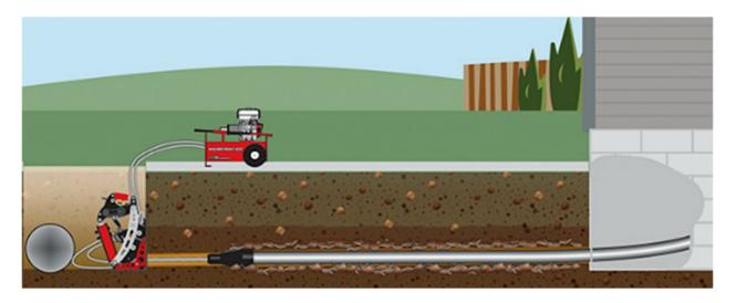
Sewer lateral lining involves injecting an epoxy resin into liner that is inserted into the damaged pipe. The liner is cured with heat or light to make it hard. While the pipe diameter is reduced slightly, the capacity of the lateral is not reduced due to the smooth interior of lined lateral.
