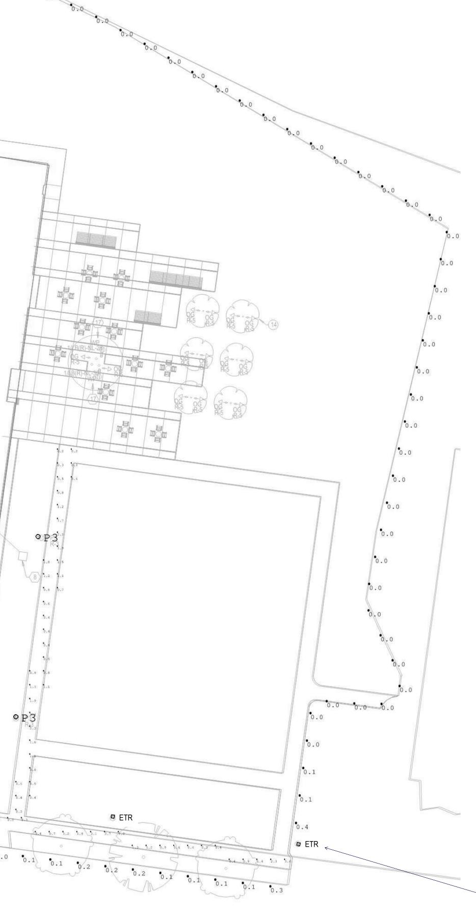
'ETR' REFERENCES EXISTING POLES ALONG SIDEWALK. NEW TYPE 'P4' TO MATCH IN STYLE
