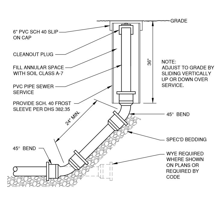
NOTE: CLEANOUT LINE TO BE THE SAME SIZE AND MATERIAL AS SEWER MAIN
