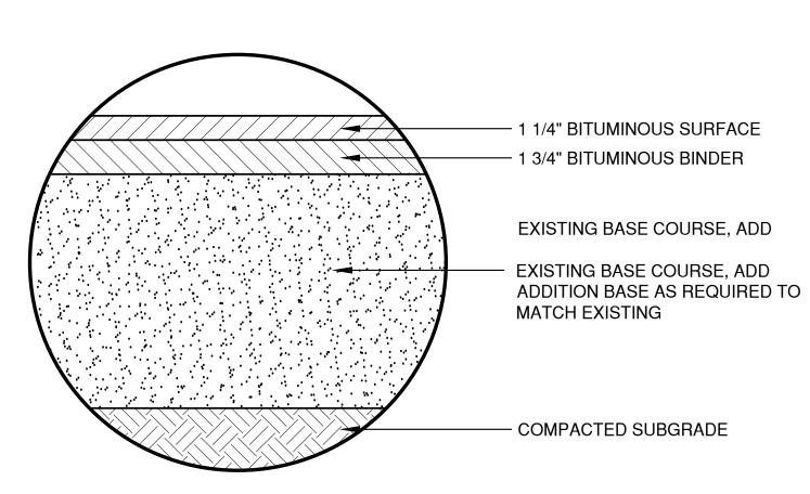
HEAVY DUTY ASPHALT PAVEMENT
