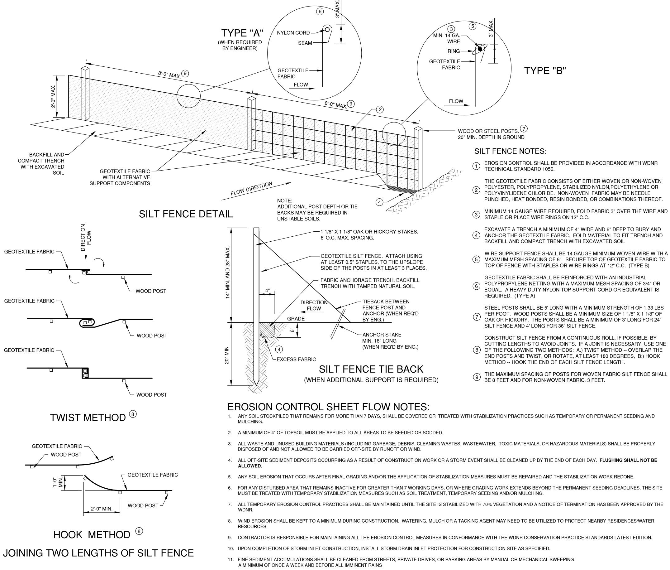
12. EROSION AND SEDIMENT CONTROL STRUCTURES SHALL BE INSPECTED WEEKLY AND WITHIN 24 HOURS OF RAINFALL OF 0.5" OR MORE
