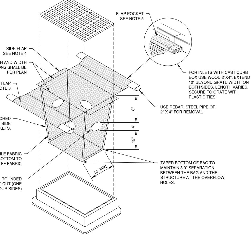
INLET PROTECTION, TYPE D (CAN BE INSTALLED IN INLETS WITH OR WITHOUT CURB BOXES)
