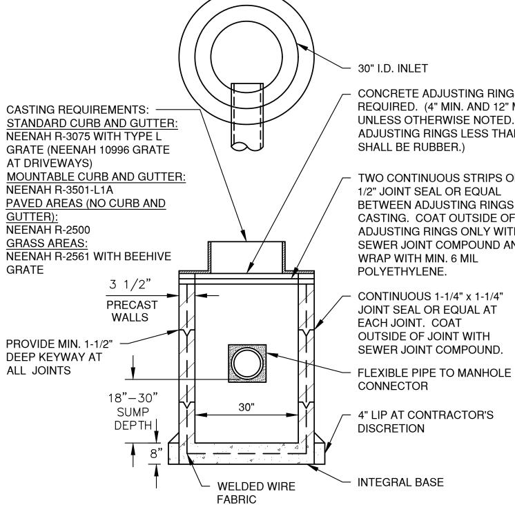
WRAP WITH MIN. 6 MIL POLYETHYLENE. CONTINUOUS 1-1/4" x 1-1/4"
