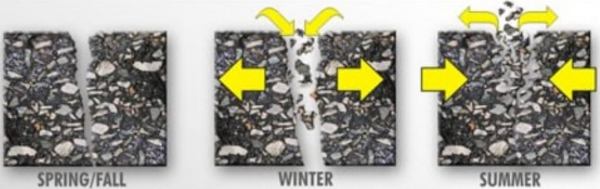
Unsealed cracks grow larger because of the intrusion of water and debris entering and then the compressive forces on the debris during the summer months.
