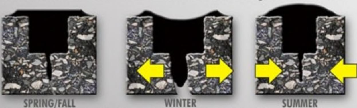
A routed crack reservoir allows for seasonal expansion and contraction of the pavement movement protecting the integrity of the sealant.
