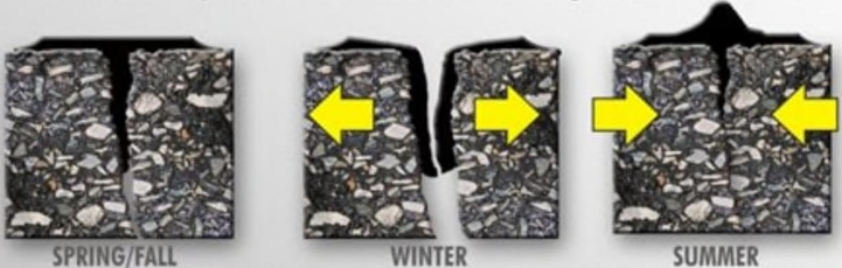
Simple crack filling exposes the sealant to traffic wear during the warm summer, the reduced amount of sealant results in cohesion failure during the winter season.
