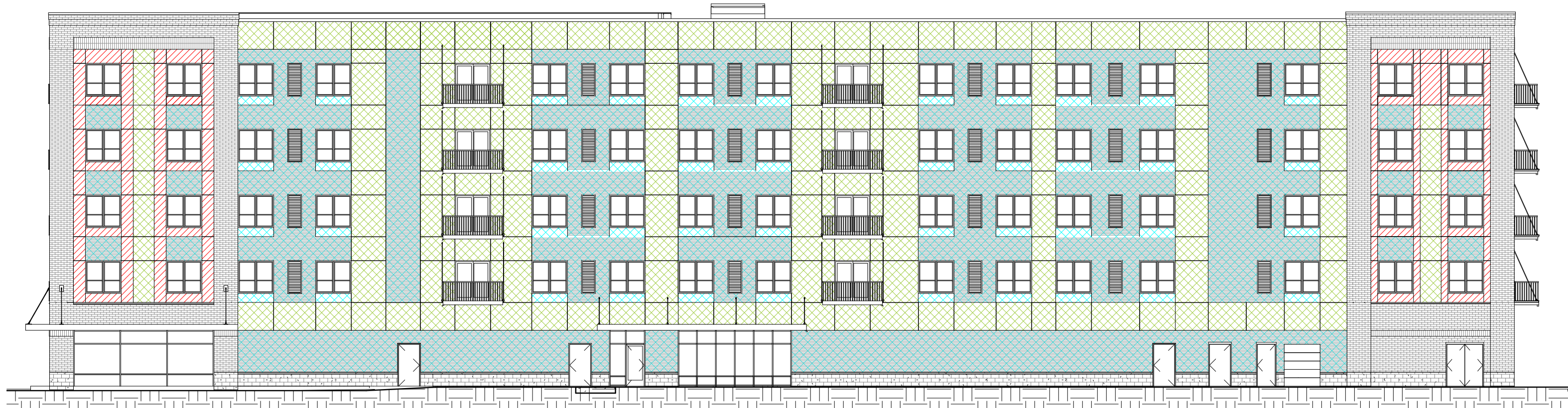
D1 SOUTH ELEVATION - METAL PANEL THICKNESS 1/16" = 1'-0" | A201
