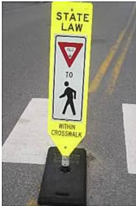
In-street pedestrian crossing signs can provide an added benefit of taming traffic speeds by creating a narrow lane perception to drivers. The estimated cost per sign is \$350.
