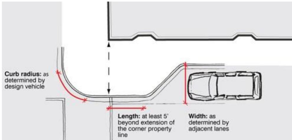
Corner curb extensions often are used to protect on-street parking areas and have the ability to provide opportunities for downtown streetscape enhancements. The cost of reconstructing existing curb radii for a corner curb extension is approximately \$15,000 per corner.
