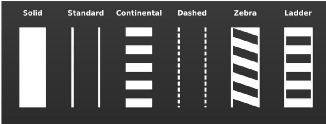
Standard Crosswalks: The standard treatment for marked crosswalks at intersections consist of two 6 to 8-inch wide white pavement marking stripes that delineate the sides of the pedestrian walking area. The stripes should be perpendicular (transverse) to the direction of vehicle travel and parallel to the direction of pedestrian travel.
