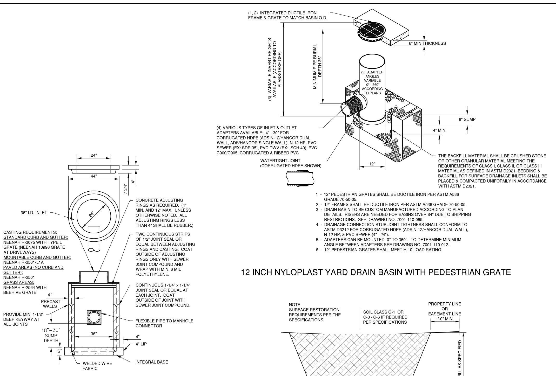
ALL PRECAST INLET UNITS SHALL CONFORM TO THE PERTINENT REQUIREMENTS OF AASHTO DESIGNATION M 199
