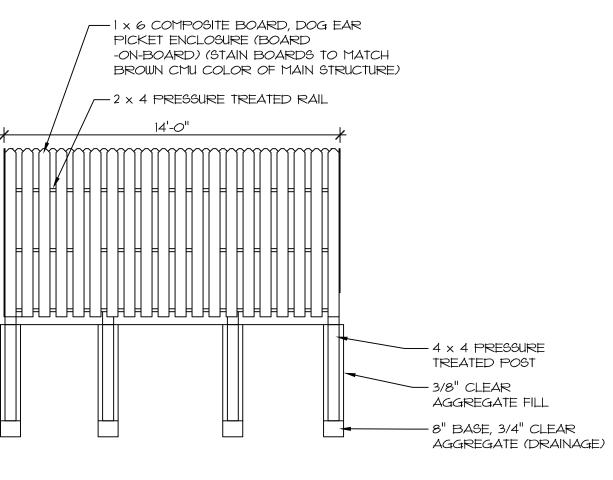
TRASH/RECYCLING ENCLOSURE EAST ELEVATION SCALE: 1/4" = 1'-0"
