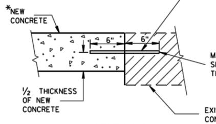
**TIE BARS DRILLED INTO EXISTING PAVEMENT**
