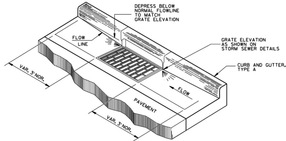
**DETAIL OF CURB AND GUTTER AT INLETS**
